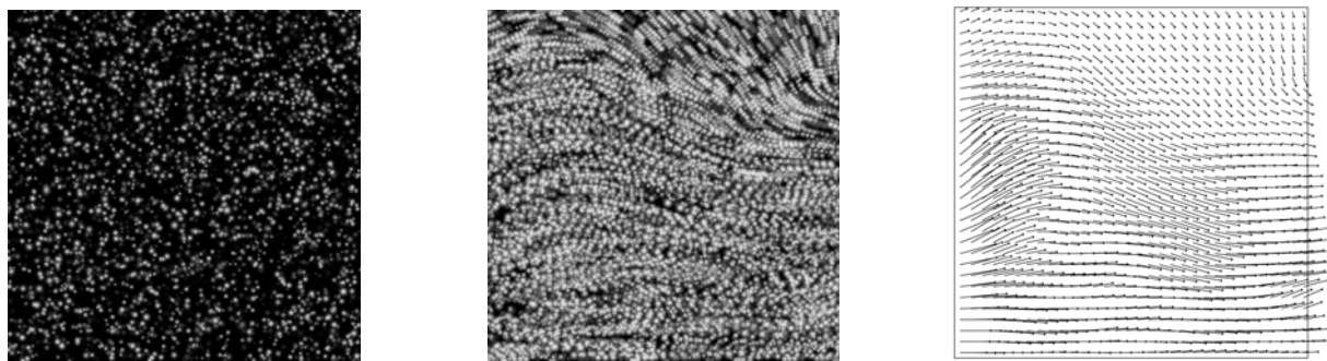
Fig. 1. One particle image, four superimposed images and the correct velocity field.
